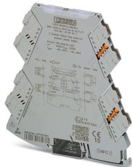
Two-channel output loop-powered 2-way repeater power supply with plug-in connection technology for the electrical isolation of analog signals. Input signal = output signal: 0(4) mA ... 20 mA. Push-in connection technology.
